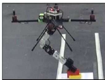
(b) Robot arm is grabbing the wood block
